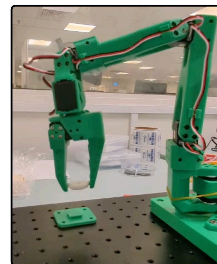
Figure 8. Waypoint Control: SO-101 performing pick-and-place of a test object
